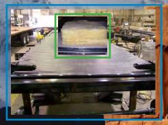
Fully Enclosed Front to Back Heated & Insulated Underbelly / Mountain Floor Insulation
