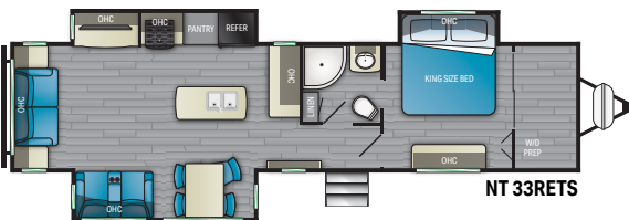
NT 33RETS Length - 39' 8" Dry - 8,840 lbs. Hitch - 780 lbs. Height - 11' 8" GVWR - 9,900 lbs.
