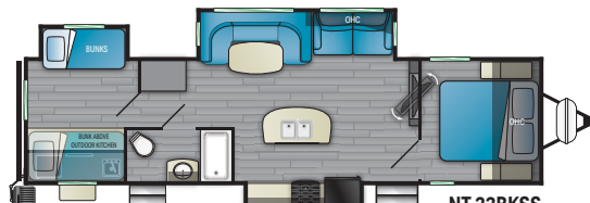
NT 33BKSS Length - 36' 10" Dry - 7,908 lbs. Hitch - 774 lbs. Height - 11' 6" GVWR - 9,600 lbs.
