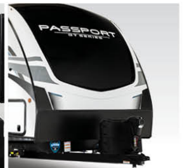
KEYSHIELD™ Automotive grade painted fiberglass front cap with chip and rock guard protection.
