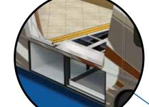
**Increased Storage:** Oversized pass-through storage re-engineered with slide rails integrated into the floor, creating more storage space and easier access.
