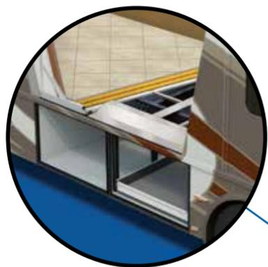
**Increased Storage:** Oversized pass-through storage re-engineered with slide rails integrated into the floor, creating more storage space and easier access.
