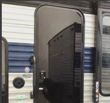
Safety Slam Friction Hinge Entrance Door
