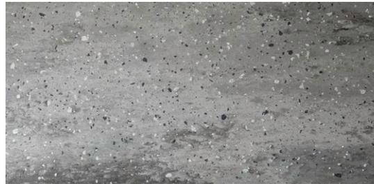
Carbon Aggregate Concrete
