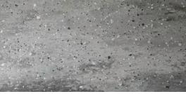
Carbon Aggregate Concrete
