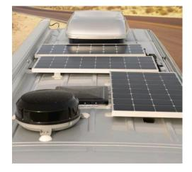
**GO POWER!® SOLAR PACKAGE** Extend your off-the-grid adventures with the addition of our solar options. This system provides power to the coach batteries, allowing for use of the 12V DC system and 120 VAC receptacles through the inverter. This gives you greater dry camping abilities without the need for shore power or running the generator. Choose from:
