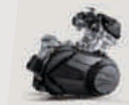
500 HO 4-VALVE, SOHC, EFI 38 HP, liquid cooled, single cylinder, 4-valve featuring Bosch® Electronic Fuel Injection and CVTech clutching.
