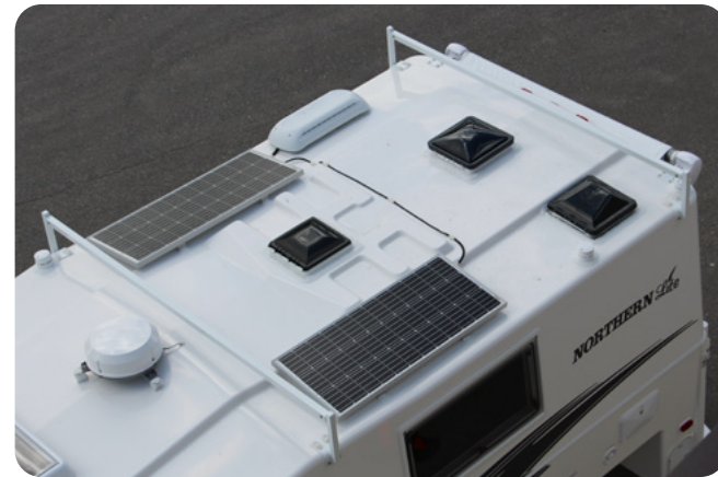
Boat Rack and Dual Solar Panels
