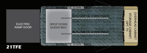
• .055 in. Aluminum Sidewall and Roof Skins Bonded • 6 in. Steel, I-beam Frame with Outriggers 7,000 lb Axle, 8 lug with Torsion Suspension 3/4 in. OSB Hi-Density Flooring with Moisture Barrier
