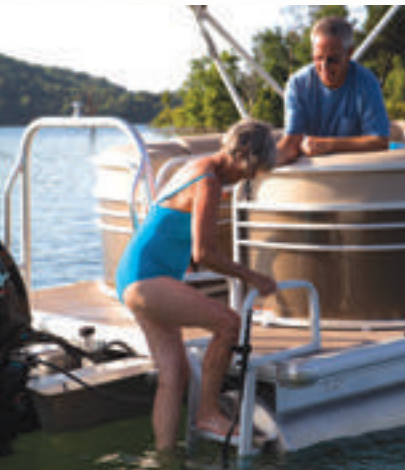
Full-width aft swim platform w/fold-down reboarding ladder
