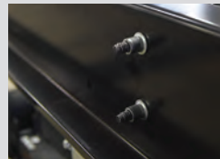
NXG Frame with Huck Bolts Adds Durability
