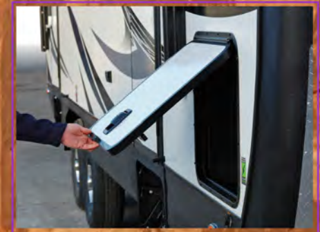
1" Thick Thermal Insulated Luggage Door Compartments
