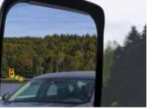
**BLIND SPOT DETECTION** (OPTIONAL) Ensure smart, safe driving with Velvac® blind-spot upgraded mirrors for your Invicta. A safety feature, where a light will illuminate on the side mirror if an object is in the blind spot ensuring safe travels. Invicta comes standard with remote power, heated mirrors with turn signals and side cameras.
