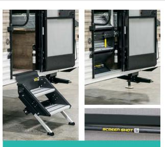
FLIP-UP ENTRY STEP and folding handrail provide solid footing and deploy effortlessly. Extra-wide 26-inch friction-hinge entry door. (Classic only)
