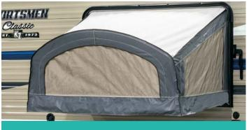
MARINE-GRADE AQUALON EDGE MATERIAL reduces heat gain by 33 percent and is permanently affixed to bunkend door. Tents feature aluminum-latched knuckle hinges, and selfsupporting cable system rated to 1,100 pounds. Aqualon Edge boasts a 7-year material warranty.
