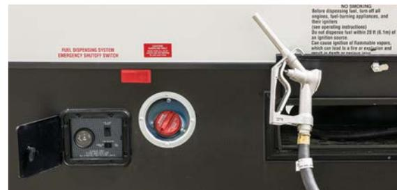
**PUMP STATION** *(Venom only, shown)* allows easy access to the 40-gallon tank. **GENERATOR PREP** includes a dedicated 30-gallon tank.
