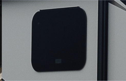
Frameless Windows Sleek and stylish windows are designed with rubber gaskets behind the glass for increased glass and seal strength.
