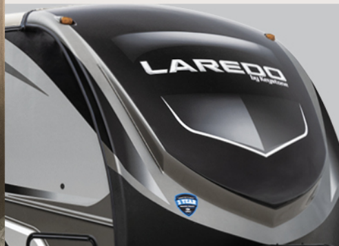
Automotive Grade Painted Fiberglass Cap Laredo caps include Keystone's exclusive KeyGuard™ protective coating, designed to provide chip and rock protection.
