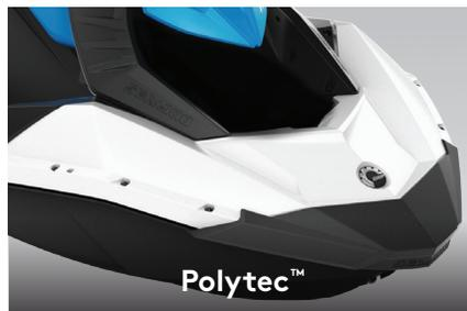
Innovative material that reduces weight while optimizing performance and efficiency. The color-in molding is more scratch-resistant than fiberglass.
