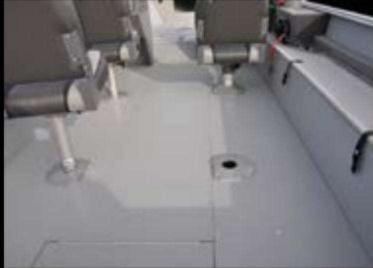
Composite flooring (Alaskan, Outfitter)
