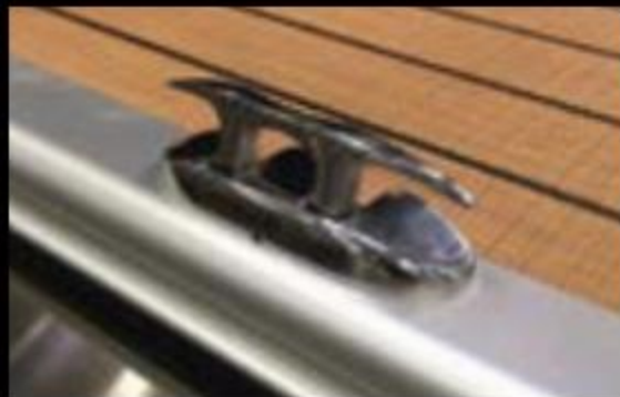
Stainless steel flip-up cleat
