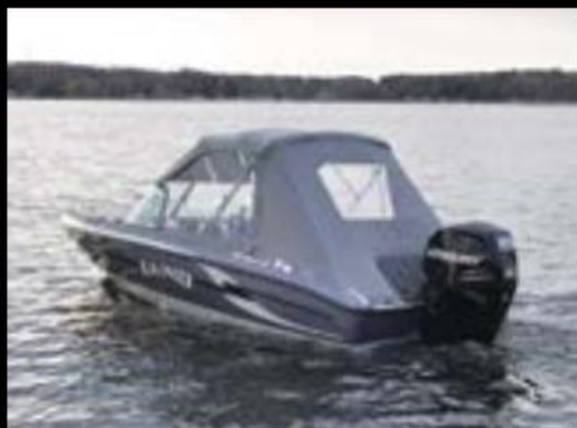
Optional full canvas *Full canvas enclosure should be used only when boat is anchored or at rest.
