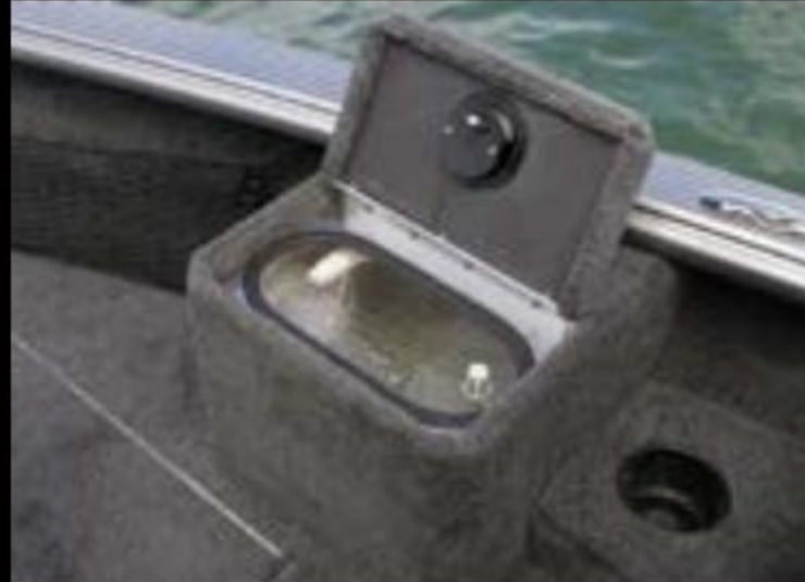
Bow baitwell (Impact / Pro-V / 1875 and 2075 Pro Guide)
