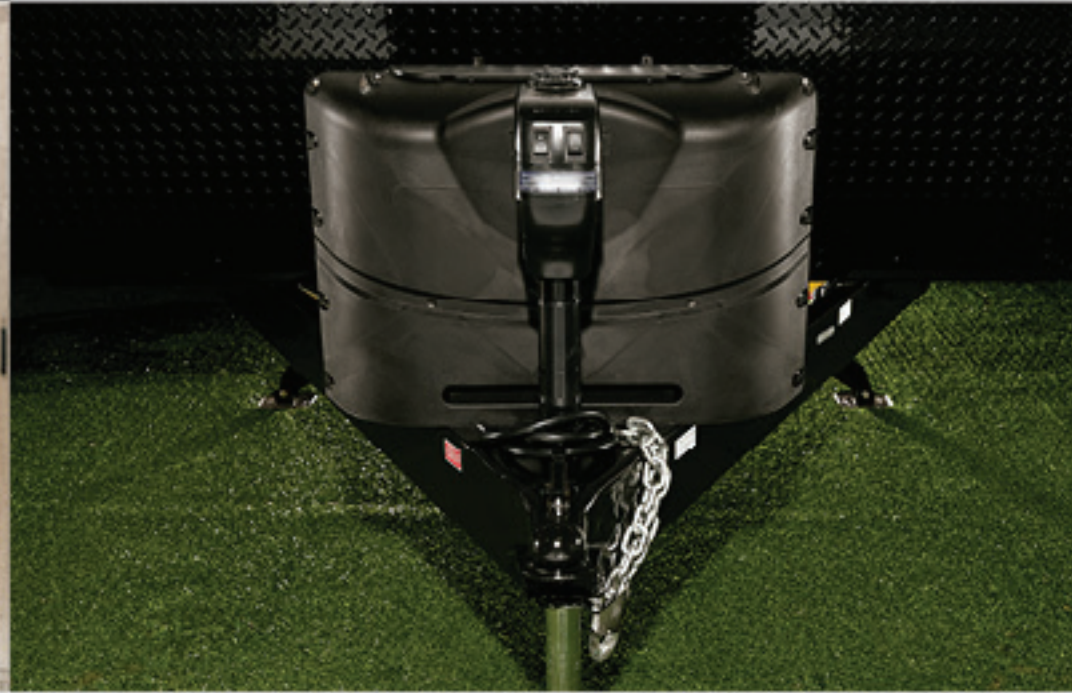
Power Tongue Jack (n/a single axle) Easy-to-use jack makes RV setup fast and simple.
