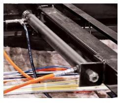
Commercial hydraulic rack & pinion slideouts. All gear boxes are located inside the frame for the ultimate weather protection.
