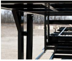
Pinless hydraulic jacks are mounted at a 5-degree angle for maximum stability.
