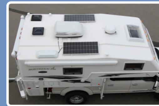
Dual 100 Watt Solar Panels on LE and SE
