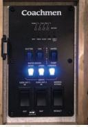
Centralized Control Panel indicates tanks, battery levels and operating components.
