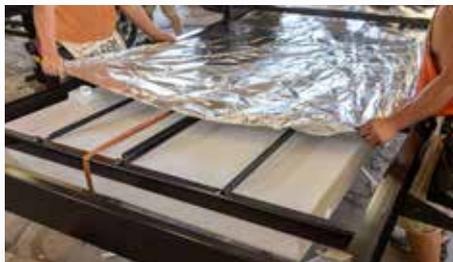
Heated holding tanks, enclosed underbelly's, larger furnaces and a radiant foil barrier in the underbelly, front cap and slide-out floors lead to a better insulated more comfortable coach year-round. (Heat pads std. Classic and Super Lite and opt. on Micro & Shamrock).
