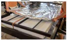
Heated holding tanks, enclosed underbelly's, larger furnaces and a radiant foil barrier in the underbelly, front cap and slide-out floors lead to a better insulated more comfortable coach year-round. [Heat pads std. Classic and Super Lite and opt. on Micro & Shamrock].
