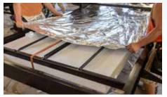
Heated holding tanks, enclosed underbelly's, larger furnaces and a radiant foil barrier in the underbelly, front cap and slide-out floors lead to a better insulated more comfortable coach year-round. [Heat pads std. Signature and Ultra Lite and opt. on Mini & Roo].
