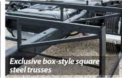
Fore and aft stringers for additional stiffness
