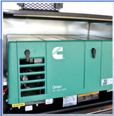
Cummins Onan 4000 Watt Gas Generator
