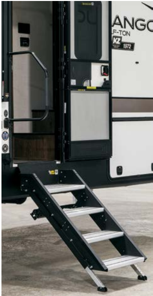
STANDARD FLIP-UP ENTRY STEP solid footing, coming and going. Handy friction hinge and screenshot auto-door-close feature.
