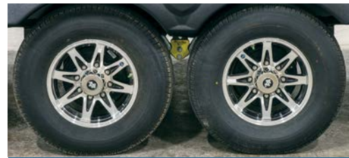
16" 6-lug heavy duty ALUMINUM WHEELS with E-range tires
