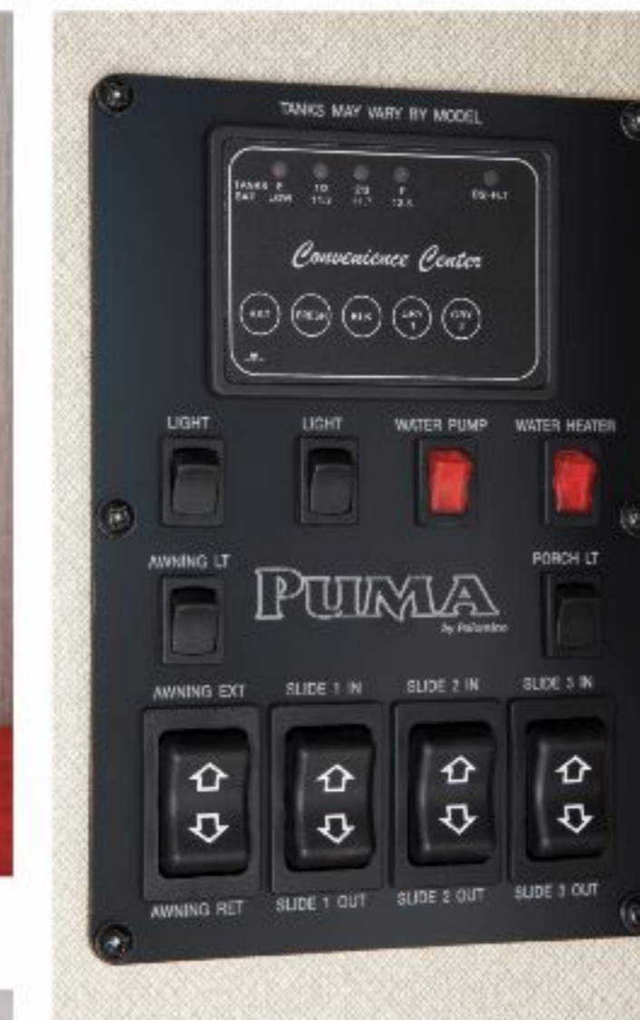
Convenience Center panel controls slides, awning, interior and porch lights, water pump/heater; shows battery/tank capacities
