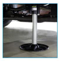
Automatic Leveling Jacks with Touch Pad Controls
