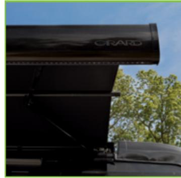
Dual Girard Roof® Mounted Patio Awnings with Integrated LED Lighting
