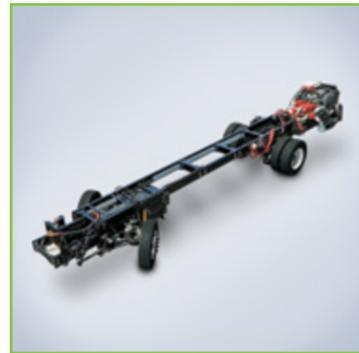
Freightliner® XC-R Raised Rail Chassis with Atlas Foundation™
