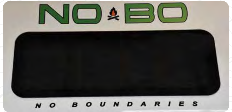
SEAMLESS PANORAMIC FRONT WINDOW 60" X 22" TEMPERED GLASS
