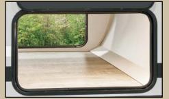
The generous cooler-sized pass-through storage compartment with magnetic catch allows for easy loading and unloading.
