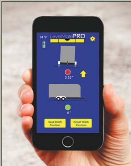
The LevelMatePRO option calculates and displays the height required to achieve a perfectly level position.
