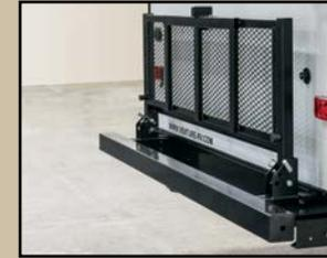
The sturdy rear rack accommodates cargo for the trip, or bicycles, and folds away completely when not in use.
