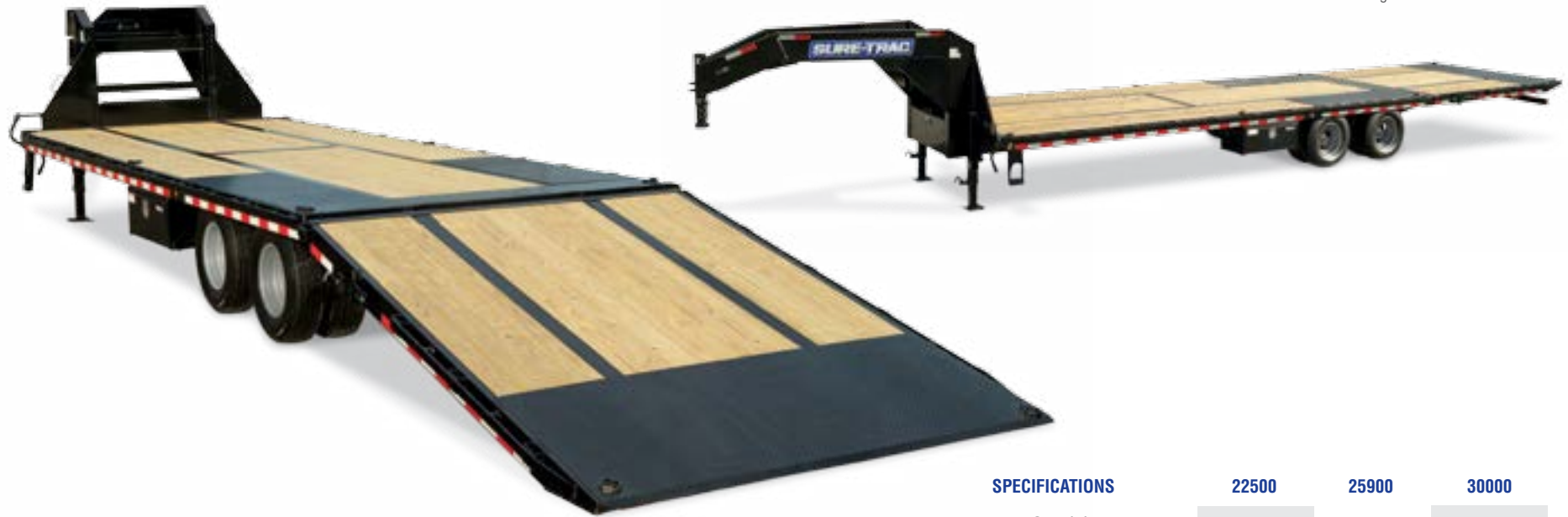
New Standard Pierced Frame for Lower Deck Height
