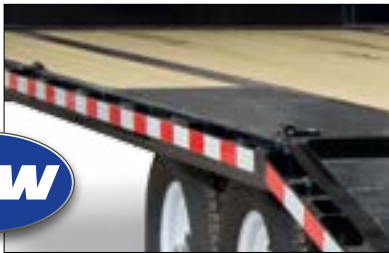
New Standard Pierced Frame for Lower Deck Height
