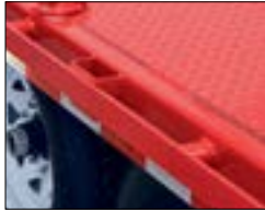
HD Stake Pockets, Rub Rail and Chain Spool
