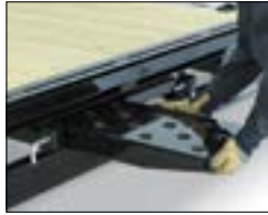
Integrated Ramp Storage
