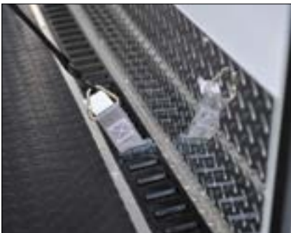
E-TRACK TIE-DOWNS AND ATP KICKPLATE
