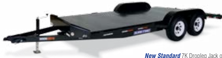
New Standard 7K Dropleg Jack on 10K Models
