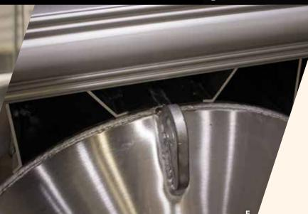
A THROUGH-BOLTED TRANSOM 1) A one-piece body with an all-welded transom is built with .190" gauge aluminum and metal boxed channel on the inner transom. A pre-drilled motor mount attached with 20 bolts allows for the heaviest high horsepower engines. 2) .190" gauge aluminum is turned down for strength and structure. 3) Spray deflectors with reinforced gussets push the water away. 4) "V" provides clean water to propeller for better turning.
