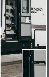
STANDARD FLIP-UP ENTRY STEP **CENTRALIZED** solid footing, coming and going. Handy friction hinge and screenshot auto-door-close feature
