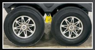
8-lug, heavy-duty, 16-inch ALUMINUM WHEELS with E-range tires (G-range on select models)
