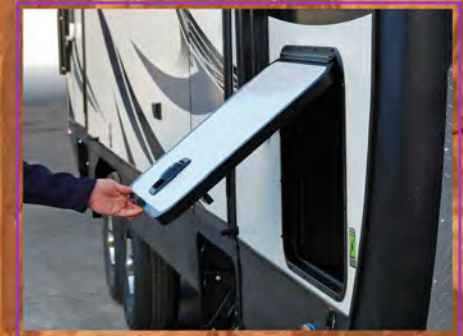
1" Thick Thermal Insulated Luggage Door Compartments
