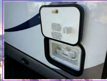
Exterior Shower Insulated by 1" Thick Thermal Insulated Luggage Door
