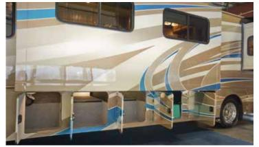
Full pass through basement storage with galvanized steel compartments and heated holding tanks.
