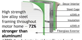
AZDEL® substrate in sidewalls and roof — No wood products!
