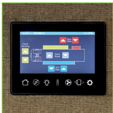
Multiplex Wiring Control System with 7" Touchscreen
