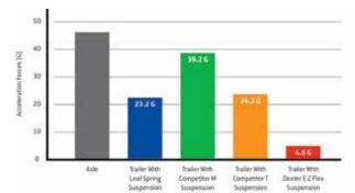
Compare acceleration forces experienced by an axle and trailer while traveling over railroad tracks at 30 MPH. The E-Z Flex® System provides up to an 80% reduction in forces on the trailer frame vs. a standard equalizer. E-Z Flex® significantly outperforms all other competitors in the same road test for a smoother, more protective ride for your trailer and cargo.
