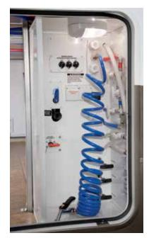
The Docking Station includes outside shower, black tank flush, water bypass, 12V battery disconnect, selector switches, dump valves, water tank and city fills for centralized convenience.
