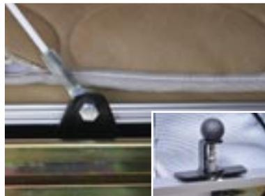
*This exclusive "Glide-N-Lock" cable supported bed system eliminates the need for support poles under the beds. Simply pull out the bed, click and it's locked into place.*
