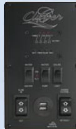
Interior Command Center controls awning, interior lighting, slide out, water heater/pump, battery indicator lights and has two USB outlets.
