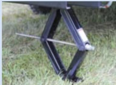
Four standard heavy duty stabilizing jacks
