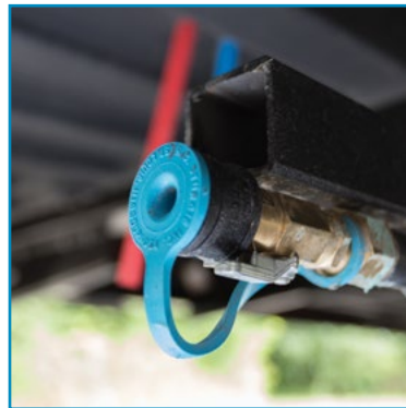
Exterior LP Connection
