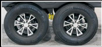
STANDARD ALUMINUM WHEELS with nitrogen-filled radial tires. (FWs only)
