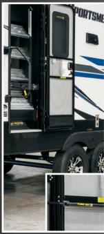
FLIP-UP ENTRY STEP provides solid footing and folds away neatly. The friction-hinged entry door with grab bar and screen-shot feature eliminates slamming, for safe and easy passage.
